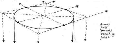
If part of the larger shape is facing the observer, some of the lines will be parallel to the picture plane and will be drawn parallel in the picture. It is worth noting that the line that is drawn horizontally through the centre of the circle will not be the longest axis of the ellipse, since the half of the circle that is nearer to you will appear larger than the half which is further away.
